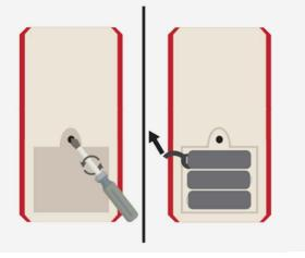
Open the battery compartment, remove the paper, secure battery in place, and screw closed.
